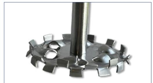
In the laboratory, dispersion of dry wax can be achieved with a disk tip speed of 1,000 – 1,500 feet per minute (FPM), or around 5 – 7 meters per second (m/s). In a production environment, a tip speed of 4,000 – 5,000 FPM, or around 22 – 26 m/s, is a good target.
